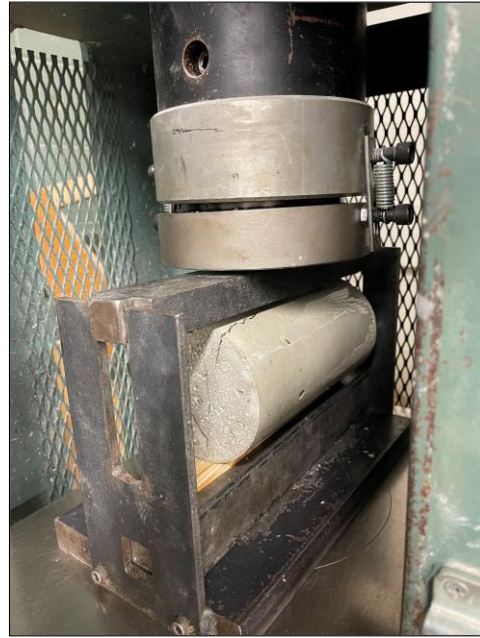
Fig 7.3. Split-tensile strength test setup
