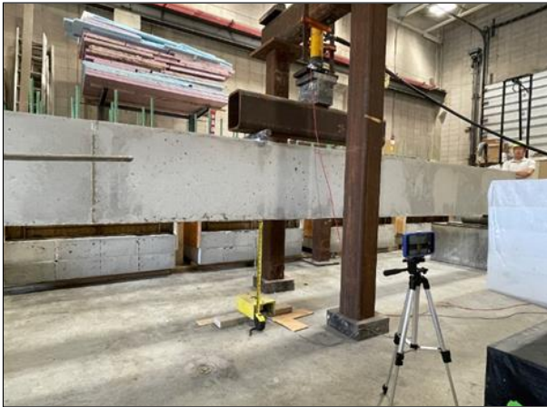
Fig 16.7. Beam setup with camera
