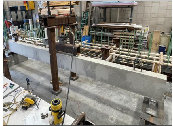
Fig 7.5. An overview of the setup for big beam testing
