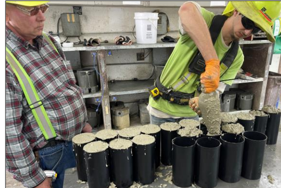
Fig 6.11. Casting concrete cylinders for strength testing
